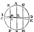
for that inftrument; namely, EF and GH, two filver wires parallel to the diameter AB, and distant therefrom 30° = AE = AG = BF = BH, the three parallel wires EF, AB, and GH, being fixed, whilft the moveable wires CD and IK
